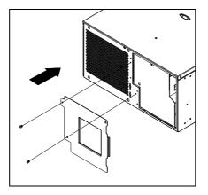
(5) Tighten the screws and replace the cable protection cover and the front panel.
